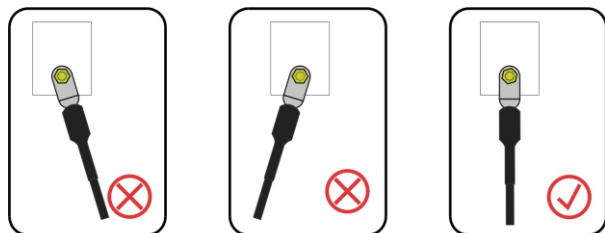
Figure 5-5 Ensuring the cables are parallel
